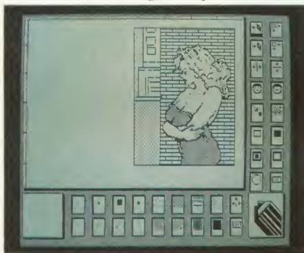
Figure 3. The studio for creating or altering pictures and headlines. Icons choose pens and fills, disc, copying and rotating facilities and pixel editor
